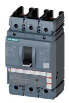
circuit breaker 3VA5 UL frame 250 breaking capacity class H 65kA @ 480V 2-pole, line protection TM210, FTFM, In=80A overload protection Ir=80A fixed short-circuit protection li=10 x In without connection
