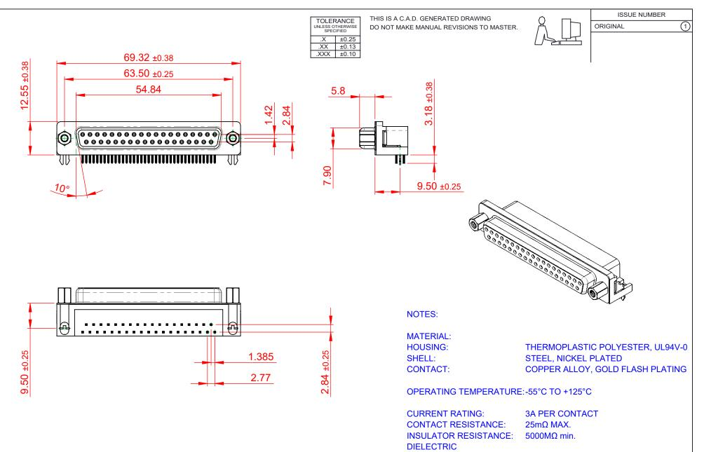
WITHSTANDING VOLTAGE: 1000V AC rms
