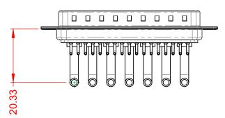
POWER/CO-AX CONTACT RATING:30A (CURRENT)(IF PRESENT)SIGNAL CONTACT CURRENT RATING:5A PER CONTACTSIGNAL CONTACT RESISTANCE: $10m\Omega$  MAX.INSULATOR RESISTANCE:5000MΩ min.DIELECTRICDIELECTRIC
