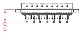
POWER/CO-AX CONTACT RATING: (IF PRESENT) SIGNAL CONTACT CURRENT RATING: 5A PER CONTACT SIGNAL CONTACT RESISTANCE:  $10m\Omega$  MAX. INSULATOR RESISTANCE: 5000MΩ min.
