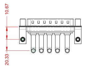
40A (CURRENT) POWER/CO-AX CONTACT RATING: (IF PRESENT) SIGNAL CONTACT CURRENT RATING: 5A PER CONTACT SIGNAL CONTACT RESISTANCE:  $10m\Omega$  MAX. **INSULATOR RESISTANCE:**
