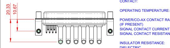
POWER/CO-AX CONTACT RATING: 40A (CURRENT) (IF PRESENT) SIGNAL CONTACT CURRENT RATING: 5A PER CONTACT
