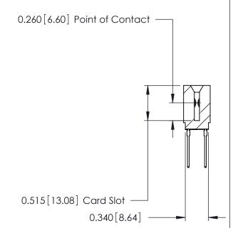
ACAD REFERENCE NO. 746-ENG MASTER 746 Series Ultra-Mate Card Edge Connector - Press Fit DRAWN: J.LEE DATE: AUG 20/09 Part Number: 746-042-540-201 CHECKED: DATE: **EDAC INC** SCALE: SHEET 1 OF 1 THESE DRAWINGS AND SPECIFICATIONS ARE THE PROPERTY OF EDAC INC.,AND TORONTO, ONTARIO SHALL NOT BE REPRODUCED, OR COPIED DRAWING NUMBER **ISSUE** CANADA OR USED AS THE BASIS FOR THE 746-ENG MASTER MANUFACTURE OR SALE OF APPARATUS YOUR CONNECTION TO QUALITY & SERVICE WITHOUT WRITTEN PERMISSION.
