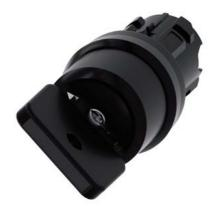
Key-operated switch O.M.R, 22 mm, round, plastic, lock number 73034, black, with 2 keys, 2 switch positions O-I, latching, actuating angle 90°, 10:30h/13:30h, Key removal O Z=50-unit packaging
