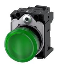
Indicator lights, 22 mm, round, plastic, green, lens, smooth, with holder, LED module, with integrated LED 110 V AC, spring-type terminal, with laser labeling, lower case
