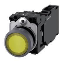
Illuminated pushbutton, 22 mm, round, plastic with metal front ring, yellow, pushbutton, flat, momentary contact type, with holder, 1 NO+1 NC, LED module with integrated LED 24 V AC/DC, screw terminal, with laser labeling, upper case and lower case, Always upper case at the beginning of the word
