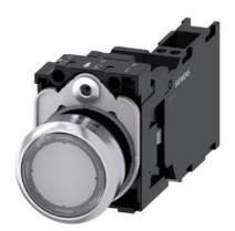
Illuminated pushbutton, 22 mm, round, Metal, shiny, transparent, pushbutton, flat, momentary contact type, with holder, 1 NO+1 NC, LED module with integrated LED 230 V AC, spring-type terminal, with laser labeling, inscription or symbol Customer-specific selection with SIRIUS ACT configurator (CIN)
