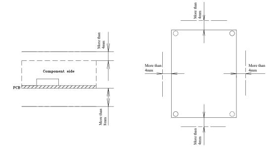
Keep 4mm space from the surfaces and sides of PCB. Especially, 8mm space is necessary from the solder surface. If the space is not enough, the specification of isolation and withstand will not be satisfied. Keep enough space in the power supply surroundings and the upper area of components for convection cooling.
