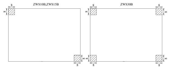
Condition to meet Isolation & Withstand Voltage standard.
