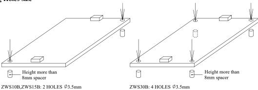
Allowable area by metal pieces is 8mm from each PCB corners. Refer to figure below.
