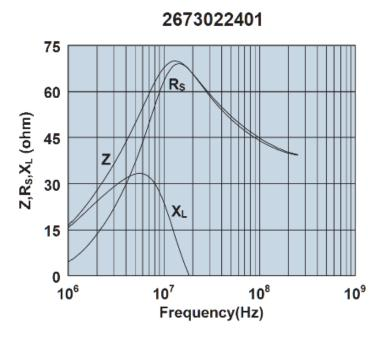
Impedance, reactance, and resistance vs. frequency.
