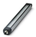
LED machine light, 24 V DC, emission angle 40 °/80 °, color temperature 5000 K, length 365 mm, diameter 40 mm, M12 connector, Light housing: Anodized aluminum, Pane: Single-pane safety glass (ESG, thermally toughened float glass), pivoting, resistant to coolants and lubricants
