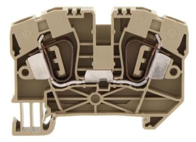
Feed-through terminal, Tension-spring connection, Mounting type: Mounting rail TS 35/7.5, Rated cross-section: 6 mm<sup>2</sup>, Width: 8.1 mm, Colour: Beige
