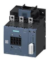
Contactor, AC-1, 275 A/690 V/40  $^{\circ}$ C, S6, 3-pole, 200-277 V AC/DC, PLC-IN optional, with varistor, 1 NO+1 NC, connection bar/ screw terminal, remaining life time
