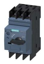
Circuit breaker size S00 for motor protection, CLASS 10 A-release 0.9...1.25 A N-release 16 A ring cable lug connection Standard switching capacity
