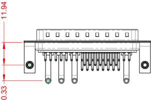
POWER/CO-AX CONTACT RATING: (IF PRESENT) SIGNAL CONTACT CURRENT RATING: 5A PER CONTACT SIGNAL CONTACT RESISTANCE:  $10m\Omega$  MAX. **INSULATOR RESISTANCE:** 5000MΩ min.
