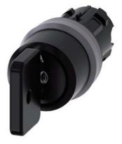
Key-operated switch O.M.R, 22 mm, round, plastic with metal front ring, lock number 73034, black, with 2 keys, 3 switch positions I>O<II, momentary contact type, actuating angle 2x45°, 10:30h/12h/13:30h, key removal O, with laser labeling, inscription or symbol Customer-specific selection with SIRIUS ACT configurator (CIN)
