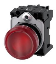
Indicator lights, 22 mm, round, metal, shiny, red, lens, smooth, with holder, LED module with integrated LED 24 V AC/DC, screw terminal, with laser labeling, upper case and lower case, always upper case at the beginning of the word
