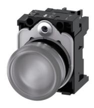
Indicator lights, 22 mm, round, metal, shiny, clear, lens, smooth, with holder, LED module with integrated LED 24 V AC/DC, screw terminal, with laser labeling, inscription or symbol Customer-specific selection with SIRIUS ACT configurator (CIN)
