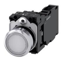
Illuminated pushbutton, 22 mm, round, Metal, shiny, white, pushbutton, flat, momentary contact type, with holder, 1 NO+1 NC, LED module with integrated LED 230 V AC, screw terminal, with laser labeling, upper case
