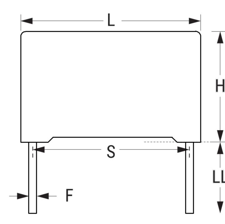
Click <u>here</u> for the 3D model. Dimensions L 18mm +0.3/-0.5mm
