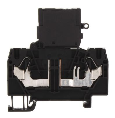
Fuse-disconnect terminal, Push-in connection, Mounting type: Mounting rail TS 35/7.5, Rated cross-section: 4 mm², Width: 6 mm, Colour: Black
