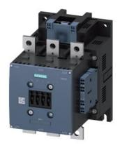
power contactor, AC-3 265 A, 132 kW / 400 V AC (50-60 Hz) / DC operation 96-127 V AC/DC auxiliary contacts 2 NO + 2 NC 3-pole, frame size S10 busbar connections drive: electronic with PLC interface 24 V DC spring-loaded terminal
