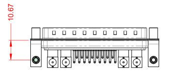
**OPERATING TEMPERATURE:** -55°C ~ 125°C POWER/CO-AX CONTACT RATING: (IF PRESENT) SIGNAL CONTACT CURRENT RATING: 5A PER CONTACT SIGNAL CONTACT RESISTANCE:  $10m\Omega$  MAX. 5000MΩ min. **INSULATOR RESISTANCE:**
