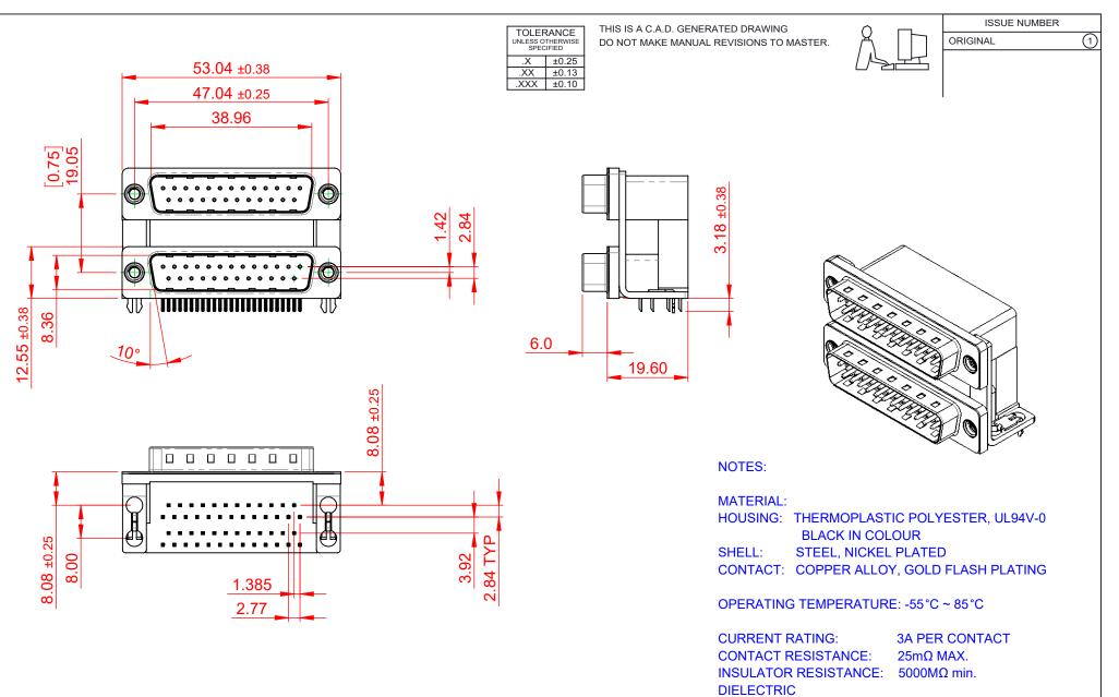
WITHSTANDING VOLTAGE: 1000V AC rms
