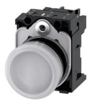
Indicator lights, 22 mm, round, plastic, white, lens, smooth, with holder, LED module, with integrated LED 24 V AC/DC, screw terminal, with laser labeling, upper case
