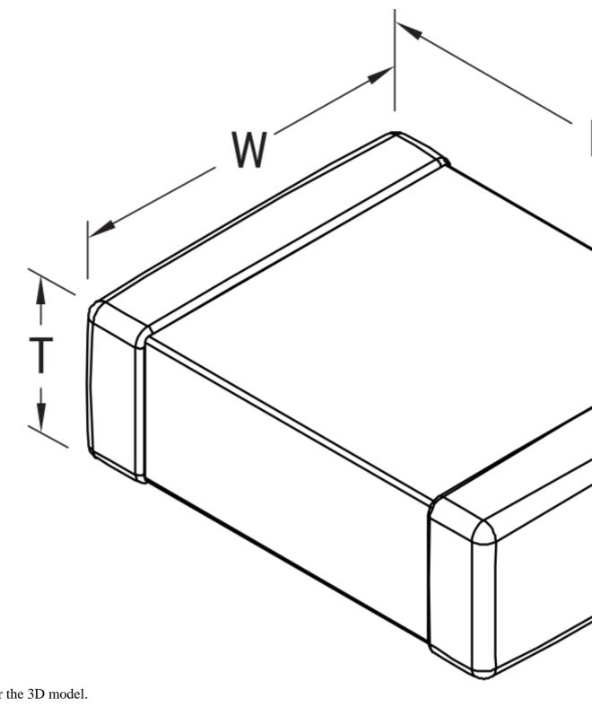
Click <u>here</u> for the 3D model. Dimensions Chip Size 1206 L 3.2mm +/-0.2mm
