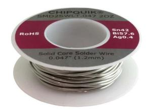
**Please Note:** Although Sn42/Bi57.6/Ag0.4 forms strong joints and is more ductile due to the added 0.4% Silver, in wire form it is brittle and needs to be handled gently when unspooling. It is normal for spooled Sn42/Bi57.6/Ag0.4 wire to have some breaks in it.
