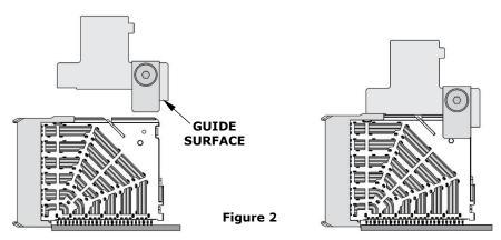
3. Using the application tool and an appropriate press, seat the Daughtercard module until there is less than 0.10mm (.004") clearance between the bottom of the plastic housing and the surface of the PCB. See Figure 3.
