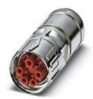
Cable connector, straight long, shielded: yes, SPEEDCON locking, M40, No. of pos.: 8+4+PE, type of contact: Socket, Crimp connection, cable diameter range: 20.5 mm ... 26.5 mm
