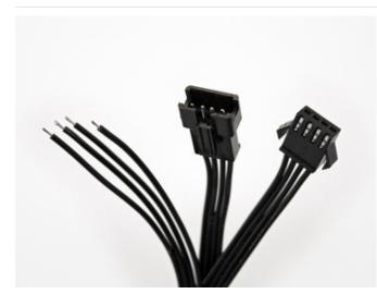
Mating connectors for both are available in the Adafruit shop. These have a housing at one end and four tinned wires at the opposite end...the wires can be soldered directly to your circuit, or strip a little more insulation to press these into Arduino pin sockets.
