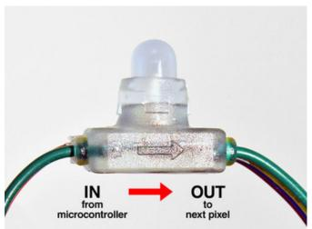
For flat pixels, look for an embossed **arrow** on the side of the plastic capsule. This represents the **direction of data flow**...bits from the microcontroller should arrive at the "tail" of the arrow, *not* the pointy head end.
