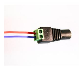
The female DC power adapter (http://adafru.it/368) mates with either of the above power supplies. Screw terminals clamp down on the power leads at the end of an LED strand, so there's no soldering required.
