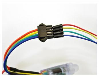
There's one more trick up our sleeve: if you don't have a mating connector available, breadboarding jumper wires can be pressed into the connector - here we're assuming that is the input side!
