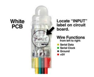
For older bullet pixels with a **white circuit board** inside, look for the "**INPUT**" label printed on the board. With this side facing you, the set of **wires in front are the input** — data arrives here — and the wires underneath are the output to the next pixel.
