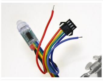
Your pixels will have one end with a plug - these tend to be the input side on **bullet** shaped pixels but we've found that isn't true 100% of the time so don't rely on this as a way of determine which end is the input
