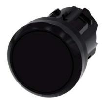
Pushbutton, 22 mm, round, plastic, black, pushbutton, flat, latching, Pushto-release mechanism, with laser labeling, inscription or symbol Customer-specific selection with SIRIUS ACT configurator (CIN)
