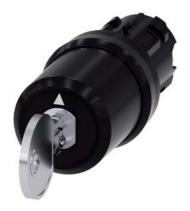
Key-operated switch BKS, 22 mm, round, plastic, lock number S1, with 2 keys, 3 switch positions I-O-II, latching, actuating angle 2x45°, 10:30h/12h/13:30h, Key removal II, with laser labeling, inscription or symbol Customer-specific selection with SIRIUS ACT configurator (CIN)
