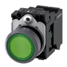
Illuminated pushbutton, 22 mm, round, plastic with metal front ring, green, pushbutton, flat, momentary contact type, with holder, 1NO, LED module with integrated LED 24 V AC/DC, spring-type terminal, with laser labeling, upper case and lower case, Always upper case at the beginning of the word
