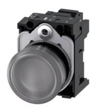
Indicator lights, 22 mm, round, plastic, clear, lens, smooth, with holder, LED module, with integrated LED 24 V AC/DC, spring-type terminal, with laser labeling, inscription or symbol Customer-specific selection with SIRIUS ACT configurator (CIN)
