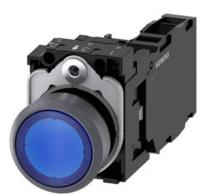
Illuminated pushbutton, 22 mm, round, plastic with metal front ring, blue, pushbutton, flat, momentary contact type, with holder, 1 NO+1 NC, LED module with integrated LED 110 V AC, screw terminal, with laser labeling, upper case and lower case, always upper case at beginning of line
