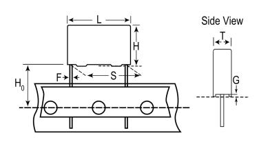
Dielectric Metallized Polypropylene Style Radial Features MKP EMI Safety RoHS Yes Lead Wire Leads Safety Class X1 Qualifications ENEC, UL, cUL, CQC AEC-Q200 No THB Performance No Component Weight 1.737 g Miscellaneous ClimCat: 40/110/56/C. Shelf Life 104 Weeks
