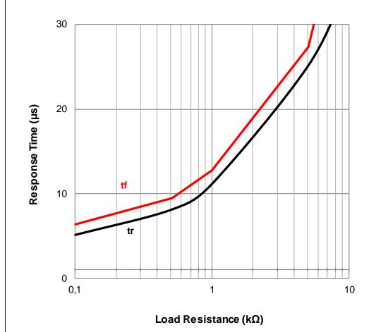
Testcondition:  $I_c = 5\text{mA}$ ;  $TA = 25^{\circ}\text{C}$
