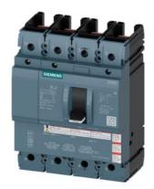
molded case switch 3VA5 UL frame 250 max short-circuit curr. rating 100kA @ 480 V 4-pole MCS110, In=150A without overload protection SELF PROTECTION Ii=16 x In w/o connection
