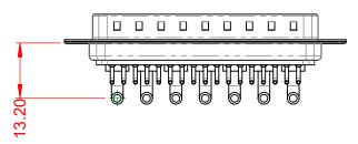
20A (CURRENT) POWER/CO-AX CONTACT RATING: (IF PRESENT) SIGNAL CONTACT CURRENT RATING: 5A PER CONTACT SIGNAL CONTACT RESISTANCE:  $10m\Omega$  MAX. INSULATOR RESISTANCE: 5000MΩ min. DIELECTRIC
