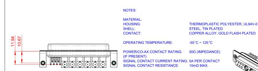
**INSULATOR RESISTANCE:** DIELECTRIC WITHSTANDING VOLTAGE: 5000MΩ min. 1000V AC rms
