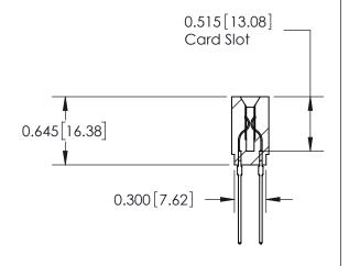
ACAD REFERENCE NO. 737 Series Ultra-Mate Card Edge Connector - Press Fit DRAWN: Part Number: 737-028-541-201 CHECKED: **EDAC INC** SCALE: THESE DRAWINGS AND SPECIFICATIONS ARE THE PROPERTY OF EDAC INC.,AND TORONTO, ONTARIO SHALL NOT BE REPRODUCED, OR COPIED DRAWING NUMBER CANADA OR USED AS THE BASIS FOR THE MANUFACTURE OR SALE OF APPARATUS YOUR CONNECTION TO QUALITY & SERVICE WITHOUT WRITTEN PERMISSION.
