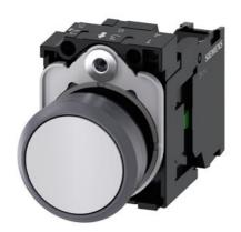
Pushbutton, 22 mm, round, plastic with metal front ring, white, pushbutton, flat, momentary contact type, with holder, 1 NO, screw terminal, with laser labeling, symbol number according to, ISO 7000 or IEC 60417
