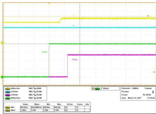
Start up with pre bias, 0 A Load Ch1: V out , Ch2:PV in , Ch3:P Good , Ch4:Enable
