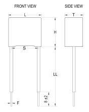
**General Information** Series R46 275 VAC Metallized Polypropylene Dielectric Style Radial EMI Safety Features RoHS Yes Lead Insulated Rigid Leads Safety Class Х2 ENEC, UL, cUL, CQC Qualifications AEC-Q200 No THB Performance No Notes We Recommended To Use R46 @ 310 VAC.
