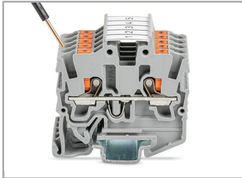
Insert solid conductors via push-in termination.
