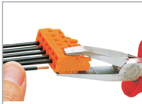
Inserting a conductor via operating tool.
