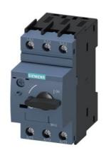
Special type Circuit breaker size S0 for motor protection, CLASS 10 A-release 27...32 A N-release 400 A screw terminal Standard switching capacity Ambient temperature -50  $^{\circ}\text{C}$  500 switching cycles
